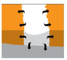
When grouting is done with a low adhering performance grouting material into the joints of impervious tiles, the adherence is much weaker resulting in grouts de-bonding from the its base.
