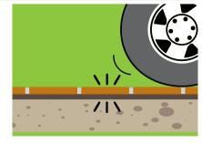
Any area of the tile grout that has no contact on the substrate and has voids under is vulnerable when subjected to a localized load. These fragile points will let cracks
