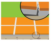
■ In case of outdoor pool and terraces; the water seeped under the covering may freeze in cold weathers. This will cause volume expansion and therefore tension under the covering. Tension may cause delaminating, cracking or deformations of the covering.
