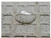
Surfaces with high absorptivity absorb the mixing water of the cementitous adhesive or other mortars very fast. Thus, the mortar loses out its mixing water and this will cause early but improper setting leading to weak adhesion and disbonding of the covering.
