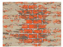
■ Loose and unstable surfaces should be removed until the sound and stable layer. Then, the substrate should be leveled with surface repairing and smoothening materials.
